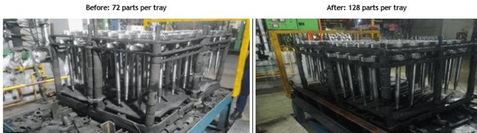
Figure 9. Tray Capacity Increase in Part No. E110
