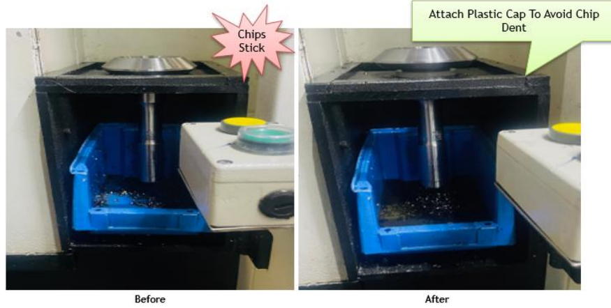
Figure 27. Metal to Metal Contact Elimination (2)
