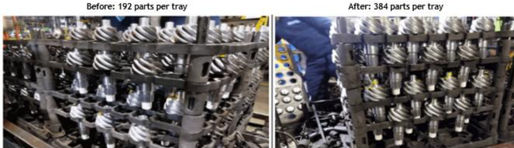
Figure 8. Tray Capacity Increase in Part No. 2804
