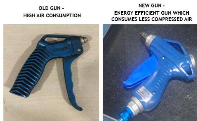
Figure 13. Installation of Air Efficient Guns to Reduce Compressed Air Consumption
