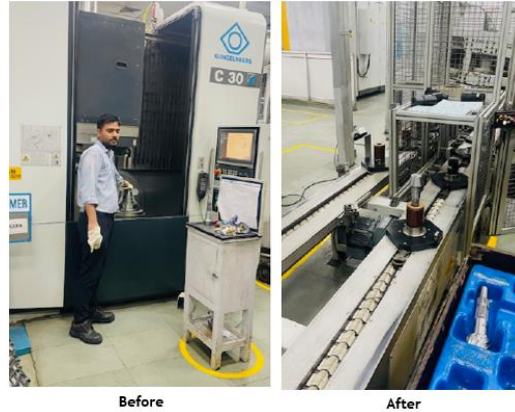
Figure 10. Autoloading Mechanism Installation
