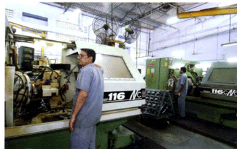
The company has horizontal CNC machines for cutting bevel gears and pinions.
