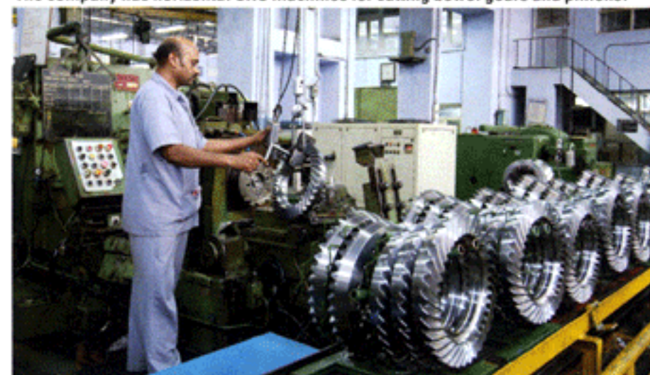
Crown gears involve precision cutting as they bear the maximum load in trucks.
